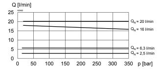
$\Delta p = f(Q)$  Pressure drop volume flow characteristic over non-return valve function of poppet valve
