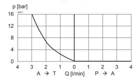
$\mathbf{Q}_{\mathrm{st+L}}$  = f (p<sub>red</sub>) Pilot- and leakage volume flow characteristice [P (2) ightarrow T (3)]
