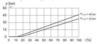
p<sub>red</sub> = f (Q) Pressure volume flow characteristics (Minimal adjustable pressure)
