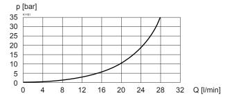
Volume flow-signal-characteristics (Δp = 10 bar) Q = f(s, x)[Type: ACB1-R] (s corresponds to preset value signal and x corresponds to spool stroke)
