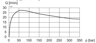
$\Delta p = f(Q)$ Pressure loss/flow characteristics (s = 100 %) [Type: ACB1-R]
