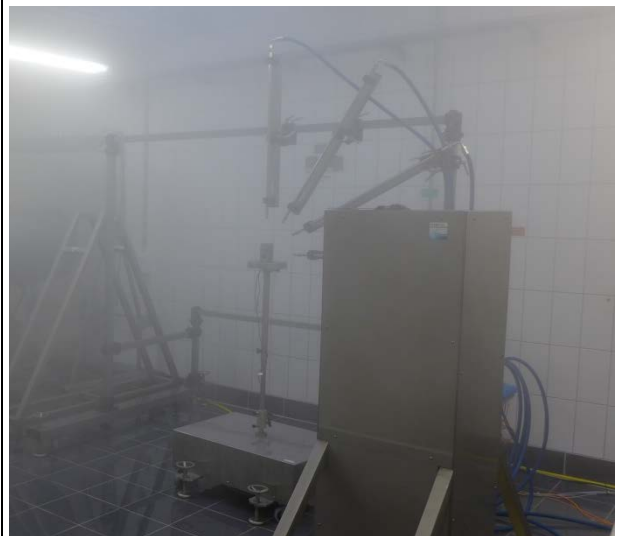
Picture shows the unit under test number 2 at the 90° angle test
