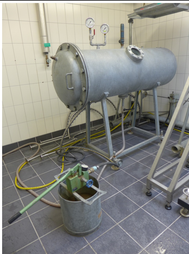
Test set up: the picture shows the pressure tank in background and in the pump in front.
