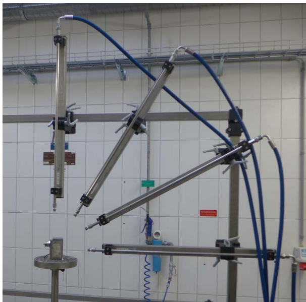
Set up position of unit under test and jets
