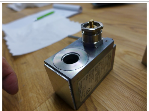
Unit under test number 2 after the 0.5 bar test.
